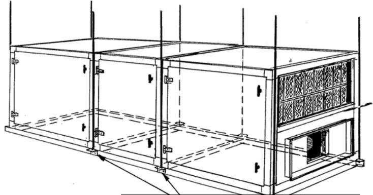
Rods connect to the framework (supplied by others) outside the unit and center with the unit section connection point.
