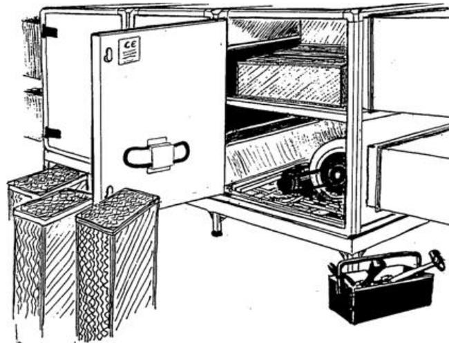
Occasionally, the heat exchanger cells may already be installed in the chamber. They must be taken out before erection of the unit and reinstalled after.
