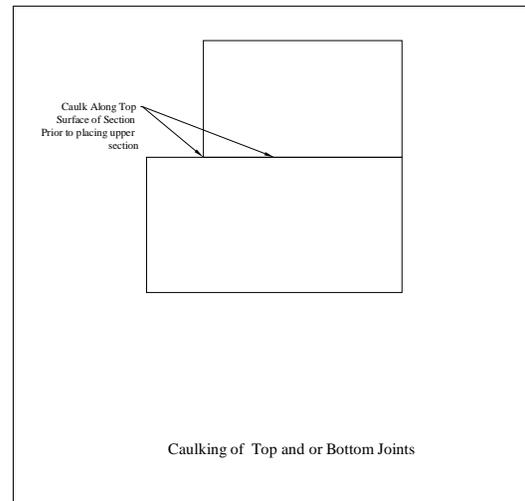
Outdoor units with sections stacked one on top of the other should be caulked prior to placing the section on the other.
