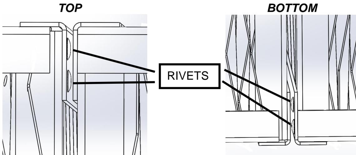
***Failure to properly align the rivets can cause the overall width of the heat exchanger cells to increase significantly. The cells will not fit in the drain pan and the door will not close!***
