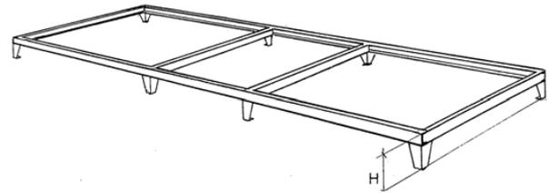
When designing the frame, the weight of the unit must be accounted for. Note that the weight of the heat exchanger cells makes the units heavier than traditional AHU's.
