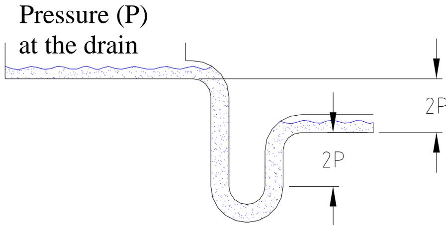
This height will also determine the height H of the mounting framework as detailed on page 6. H should be 4P, plus 2".
